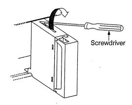
2. Push the unit in the direction of the arrow and mount onto the motherboard.
