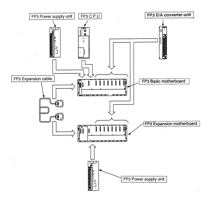
The figure above shows the system configuration.
