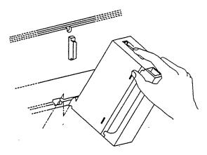
3. After properly mounting the unit to the motherboard, secure the mounting screw at the top.
