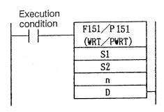
S1: D/A converter unit mounted slot
