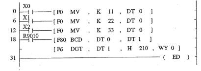
Transfers K11 to DT0 Transfers K22 to DT0 Transfers K33 to DT0 Converts the data in DT0 to BCD and stores it to DT1. Transfers data in DT1 to Y8~YF
