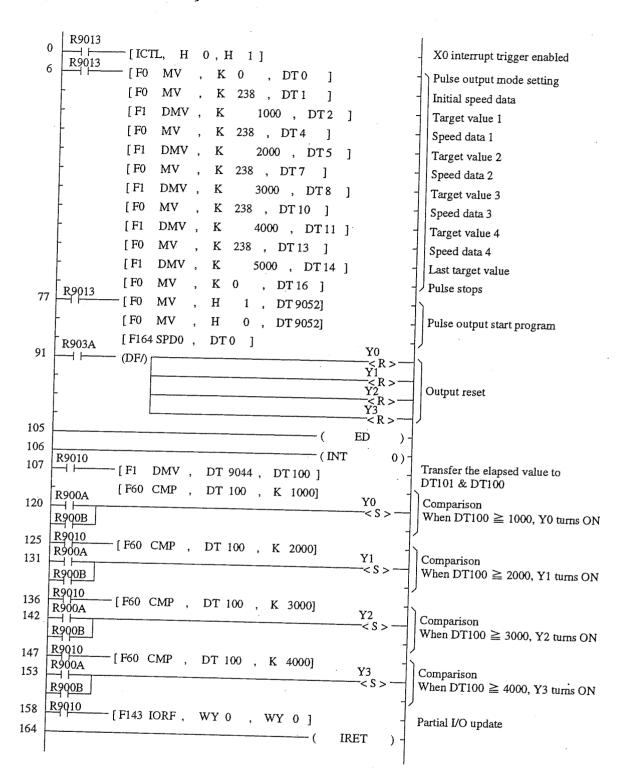
• To use the high-speed counter-initiated interrupt, first you need to set system register 400. (You do not have to set system register 403.)
