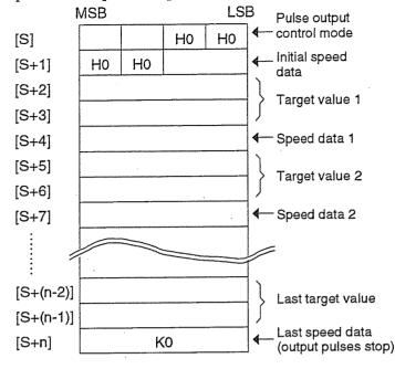
① Pulse output control mode setting Selects the frequency range and the outputs used for the instruction using hexadecimal data as follows:
