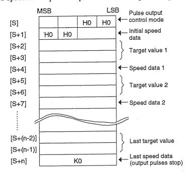
S specifies the pulse output control mode, pulse output frequency and target value as follows:
