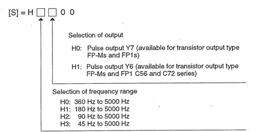
Speed data (output pulse frequency) setting Use the speed data to specify the output pulse frequency for the pulse output.
