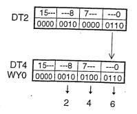
Hexadecimal digit position 0 of DT2 is transferred to the hexadecimal digit position 0 of DT4 and WY0.
