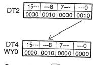
Hexadecimal digit position 0 of DT2 is transferred to the hexadecimal digit position 2 of DT4 and WY0.
