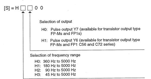
② Speed data (output pulse frequency) setting Use the speed data to specify the output pulse frequency for the pulse output. Speed data specification range: K0 to K255 The speed data can be set using the following method
