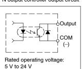
Photo-mos controller output circuit
