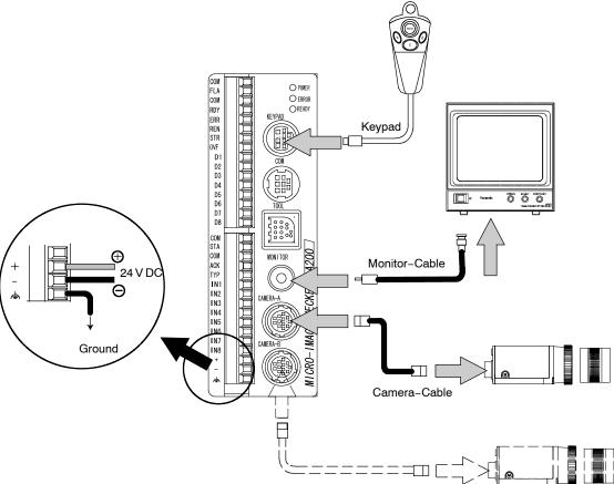
\*Only one camera can be connected to the A100.
