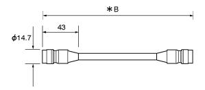
\*B is the length of the installed cable.
