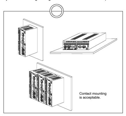
Do not mount the unit on top of strong heat sources such as heaters, transformers, or high-capacity resistors.
