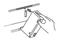
3. After properly installing the unit, tighten the screw at the top.
