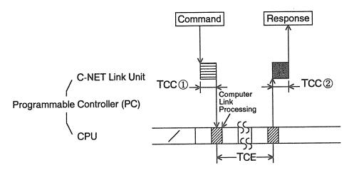
TC-NET [ Processing time needed by the Programmable Controller ] = TCC ① + TCE + TCC ②
