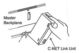
2. Push the unit in the direction of the arrow to install it in the Master Backplane.
