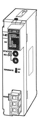
The FP3 C-NET Link Unit enables communication between Programmable Controllers (PCs) and a computer. The C-NET Link Unit is installed on a Master Backplane in the FP3 Programmable Controller (PC) and is connected to a computer and other C-NET Link Units or C-NET Adapters through an RS485 serial communications port.
